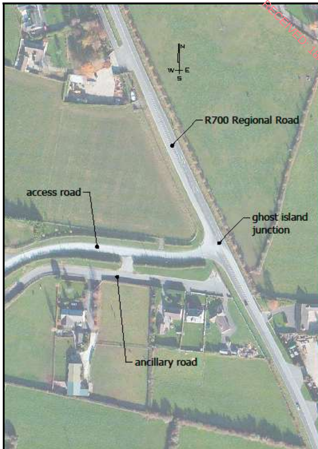
Figure 12.5.2 Access Road, Ancillary Road* and Ghost Island Junction
